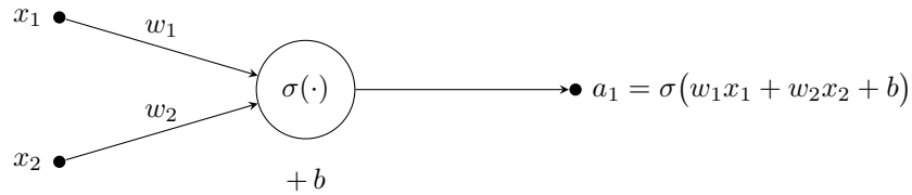
Figure 1: A single artificial neuron: it applies an activation function \sigma(\cdot) to the weighted sum w_1x_1 + w_2x_2 of its inputs plus an offset term b , and delivers the output a_1 . The weights w_1 , w_2 and the offset b are tunable model parameters. This neuron appears as node a_1 of the ANN in Fig. 2, which does not draw the offset terms
